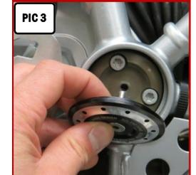
5. Refer to **PIC 3**. Attach the Plug to the bike by threading the screw into the center hole; rotate the Plug to your liking, then tighten the screw.
