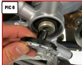
**NOTE:** Threadlocker has been pre-applied to the screws. Threadlocker (Loctite 242 or equivalent) must be re-applied if the Swing Arm Pivot Plugs are removed, then reinstalled. Follow the manufacturer's recommendations for proper thread preparation and application.
