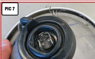
9. Remove the bulb housing from the bezel; set the bezel aside, it will not be reused.
