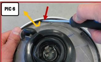
Press one of the spring legs down and under the bezel lip.
